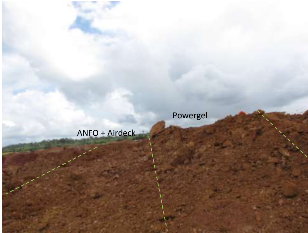
Figure 2: Muck pile of the SM test, notice the boulders ranging from 80 cm to 40 cm in the row of holes that was loaded with powergel. The finely fragmented ore on the left was the result of a airdeck and ANFO.
