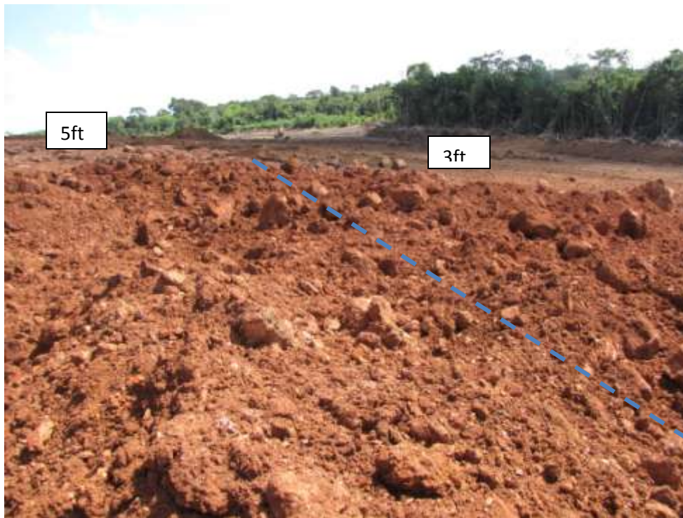
Figure 1: Muckpile of CBO Blast. Maximum boulder size of 50-60 cm, ratio of finely fragmented ore to boulders was 85-15 percent approx. best results achieved with the 5ft stemmed holes.
