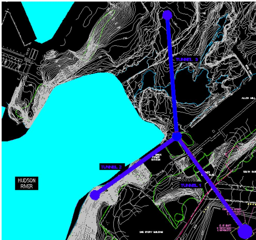
*Figure 3 – Plan view of the TDCS Shaft and Tunnels*
