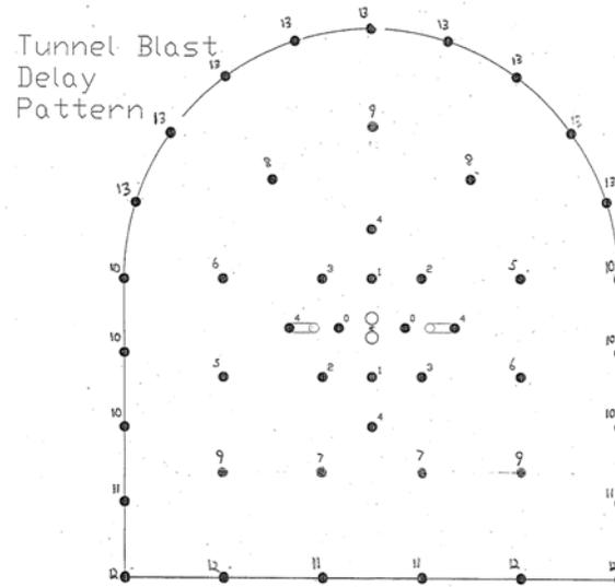
*Figure 6 – Typical tunnel blast design*
