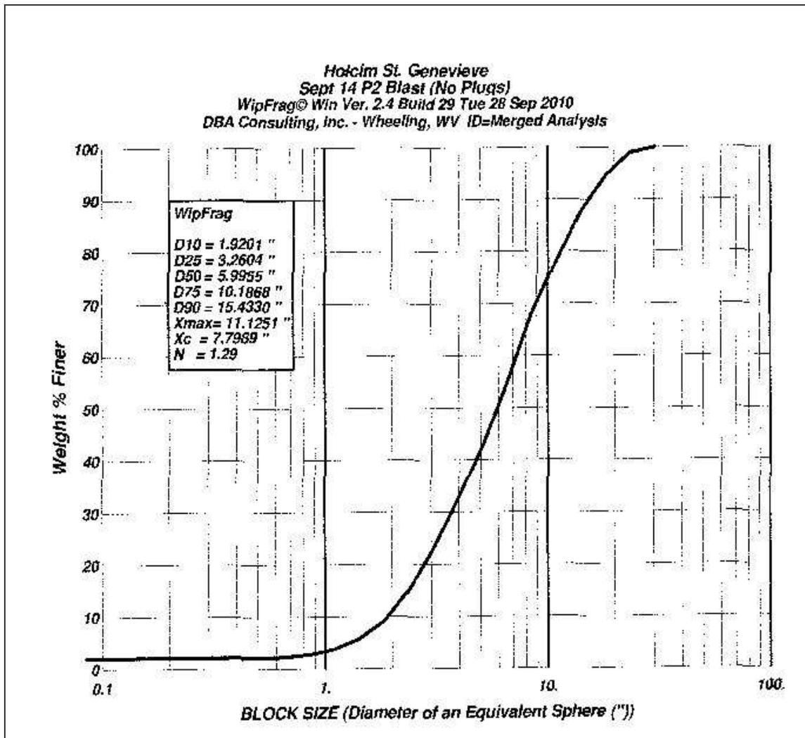
Distribution curve of fragmentation analysis with no plugs used in blast holes.
