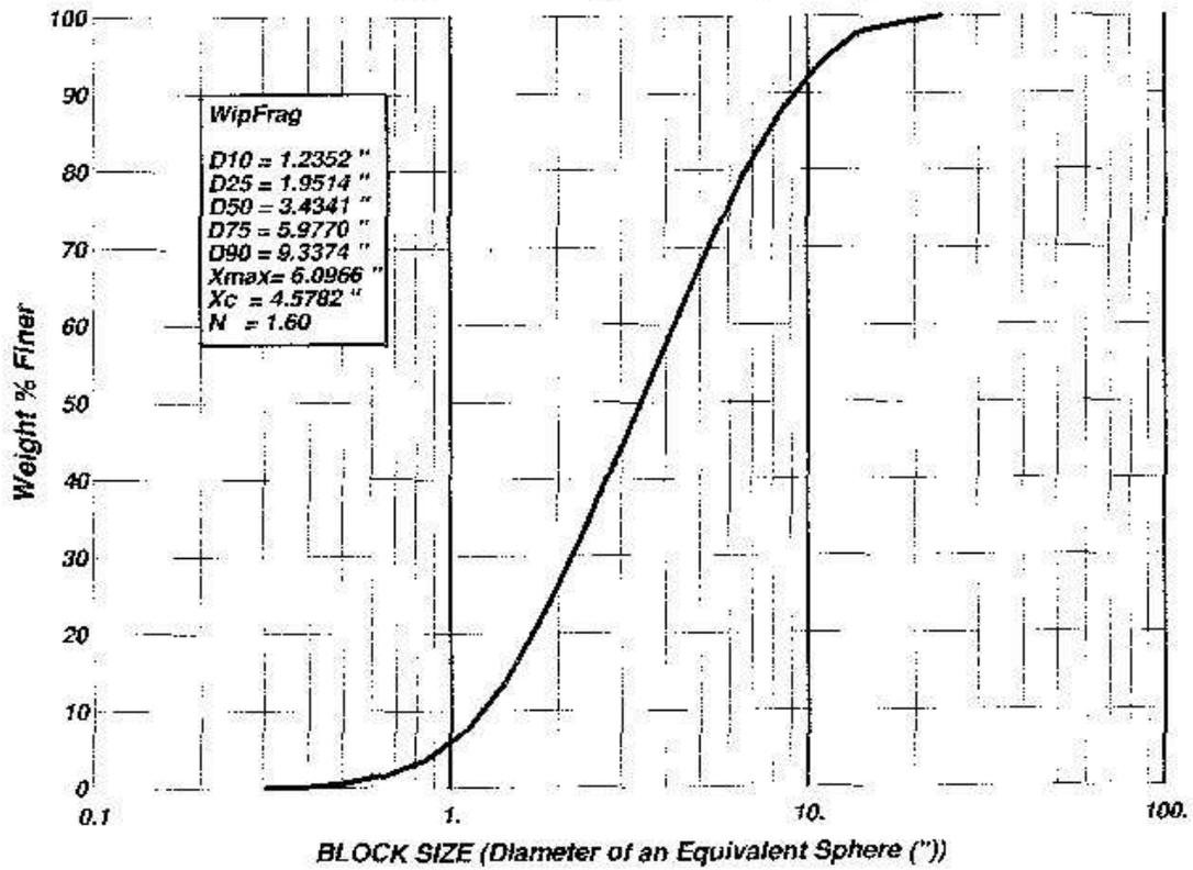
Distribution curve of fragmentation analysis with Varistem plugs used in blast holes.
