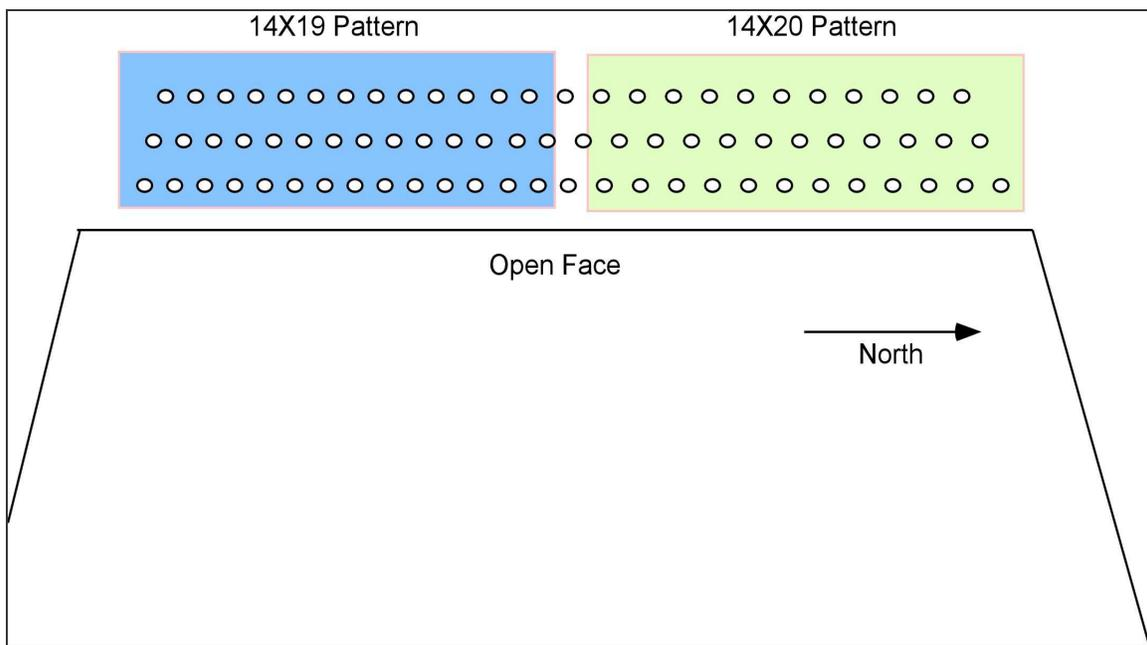
All of the blast holes in this blast were loaded using the Varistem hole plug. The fragmentation analysis was completed by sampling the muckpile at locations containing the rock from the second and back row of the blast. This was done to exclude the oversize material that typically originates from the face row of a blast from the preconditioning of the prior blast.
