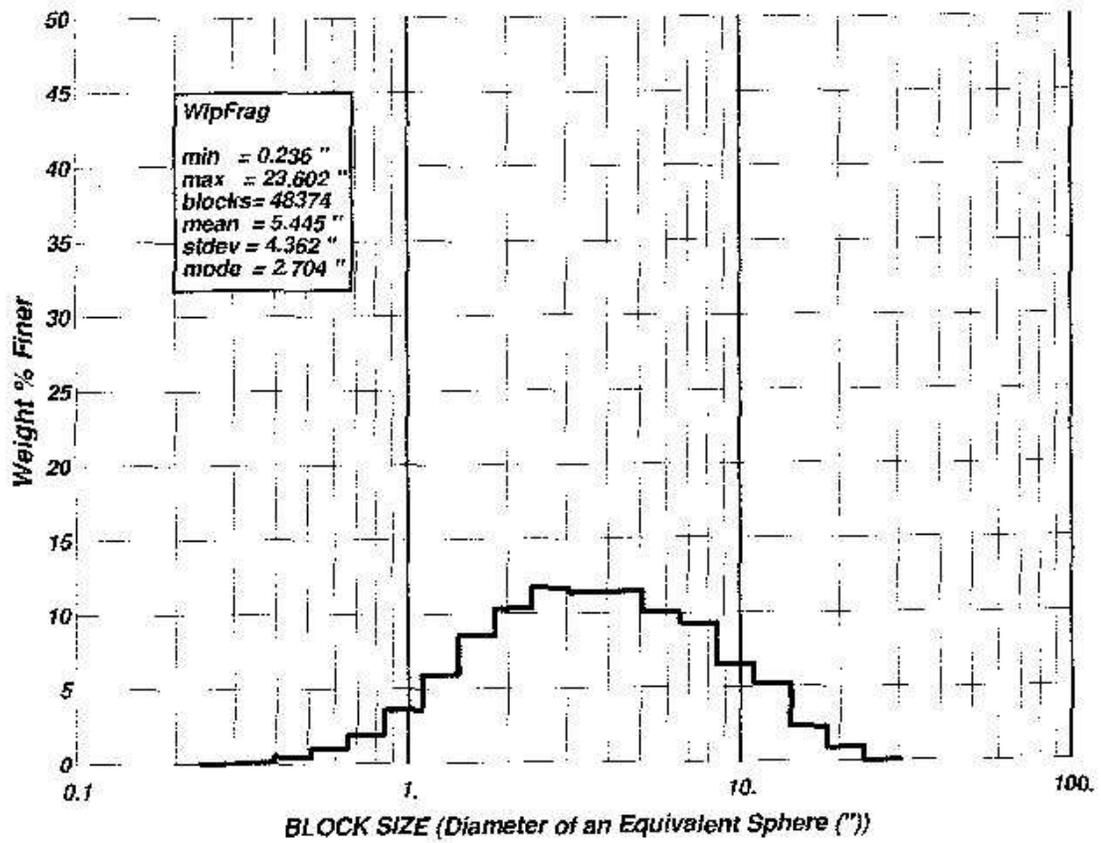
Histogram curve of fragmentation analysis with no plugs used in blast holes.
