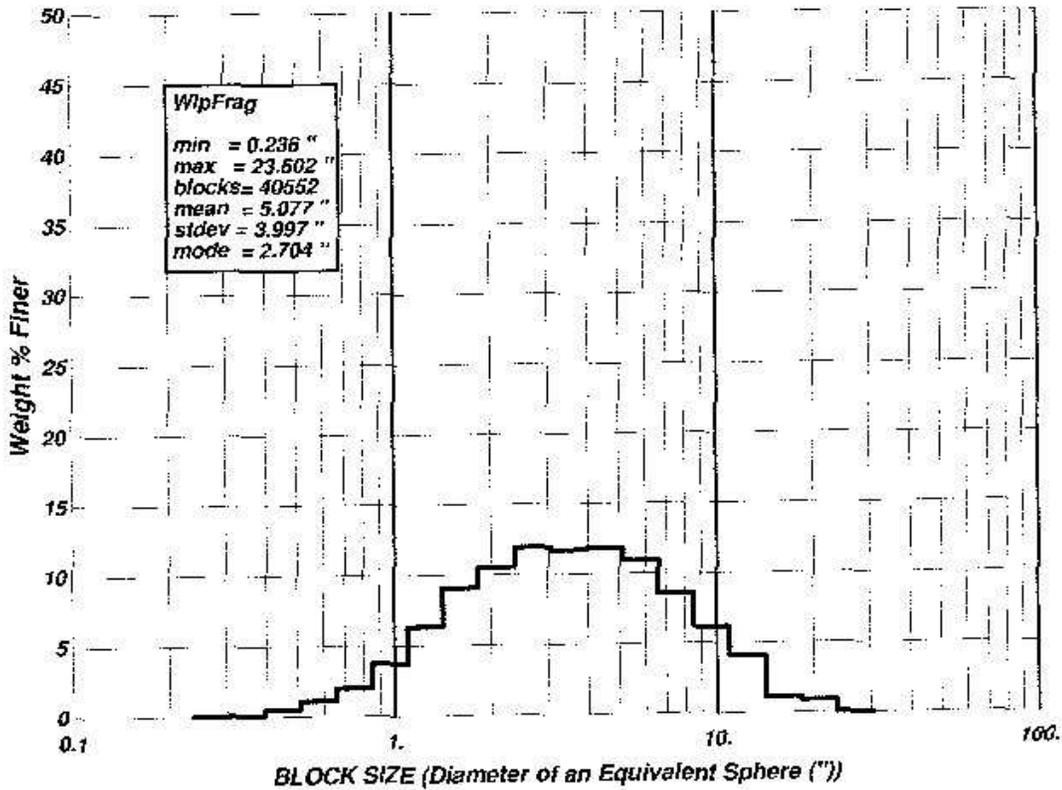
Histogram curve of fragmentation analysis with Varistem plugs used in blast holes.
