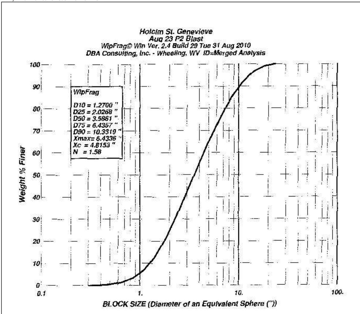
Distribution curve of fragmentation analysis with no plugs used in blast holes.
