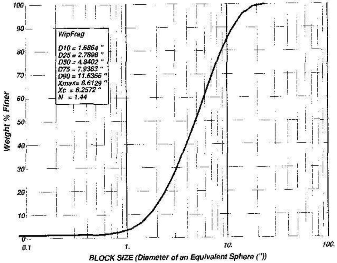
Distribution curve of fragmentation analysis with Varistem plugs used in blast holes.
