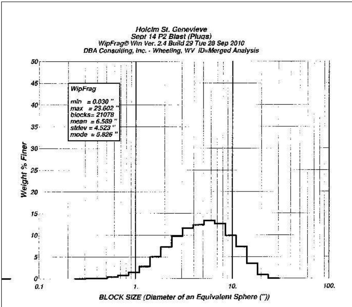
Histogram curve of fragmentation analysis with Varistem plugs used in blast holes.
